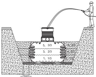
When installing the tanks in an **area to be traversed by light traffic (passenger cars)** there must be a final **bearing layer of coarse gravel** approximately 200 mm to 300 mm deep. The area of the bearing layer of coarse gravel must be equivalent to the base of the excavation.
